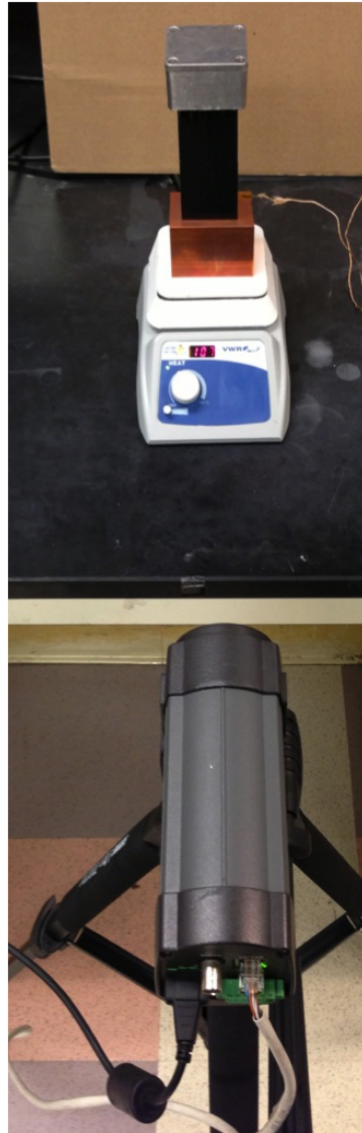
Figure 4.4: Experimental setup showing an FLIR A320 camera being used to measure temperature profiles of an experimental setup
