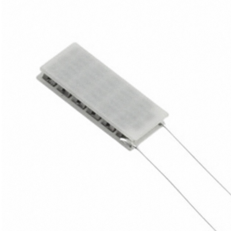
Figure 7.7: One of the TEGs used in our experiments
